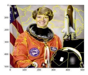
**Explanation:** We cluster the image into 100 segments with compactness = 1 and this segmented image will act as a labeled array for the mark\_boundaries() function. Each segment of the clustered image is differentiated by an integer value and the result of mark\_boundaries is the superimposed boundaries between the labels.
