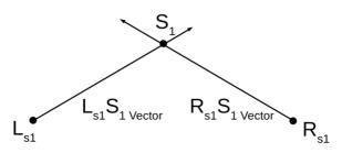
In the above figure, the direction vectors from the left and right images (Ls1S1 and Rs1S1, respectively) intersect at the single source S1. This 3D source point in the scene is the point from where light rays cast image pixels Ls1 and Rs1 in the left and right images.
