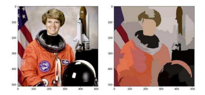
**Explanation:** This technique creates superpixels by grouping pixels in the picture plane based on their color similarity and closeness. This is done in 5-D space, where XY is the pixel location. Because the greatest possible distance between two colors in CIELAB space is restricted, but the spatial distance on the XY plane is dependent on the picture size, we must normalize the spatial distances in order to apply the Euclidean distance in this 5D
