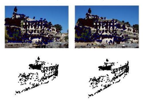
Figure 5.8: Example of computing a 3D reconstruction from a pair of images using image matches. (top) the two images with feature points shown in red and reprojected reconstructed 3D points shown in blue. (bottom) the 3D reconstruction.
