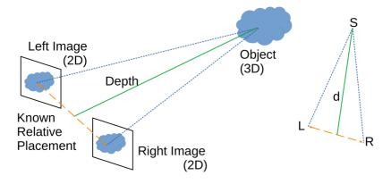
To determine the depth of S in the composite 3D image, we first find two pixels L and R in the left and right 2D images that correspond to it. We can assume that we know the relative positioning of the two cameras. The computing system estimates the depth d by triangulation using the prior knowledge of the relative distance between the cameras.
