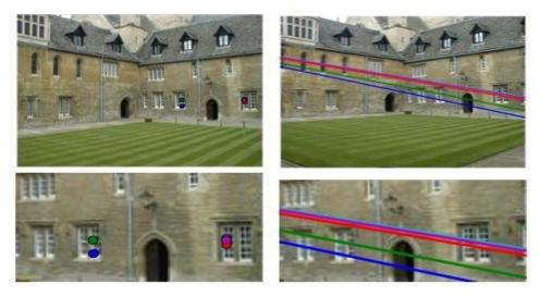
**Figure 5.4:** Epipolar lines in view 1 shown for five points in view 2 of the Merton1 data. The bottom row shows a close up of the area around the points. The lines can be seen to converge on a point outside the image to the left. The lines show where point correspondences can be found in the other image (the color coding matches between lines and points).
