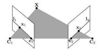
Figure 5.1 Epipolar geometry
